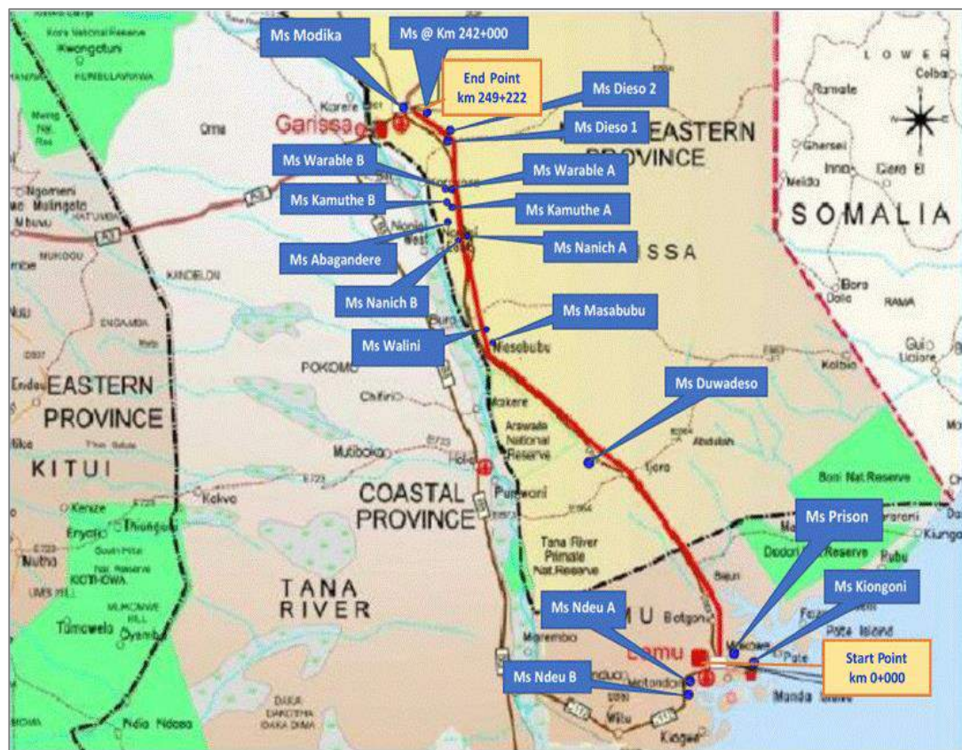
Figure 4.5 : Schematic Diagram of Sources of Embankment Soil, Subgrade and Gravel Material
